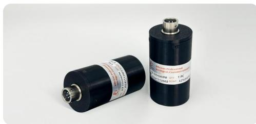
The ECB-D25H25SIPM01 spectroscopic detector is a highly integrated detector containing a 1-inch CeBr<sub>3</sub>, silicon photomultiplier (SiPM), summing circuit, preamplifier circuit, and temperature measurement circuit. It features excellent energy resolution, simple operation, compact size, and high reliability. It is widely used in industrial detection, radiological medicine, radiation detection, and other fields.
