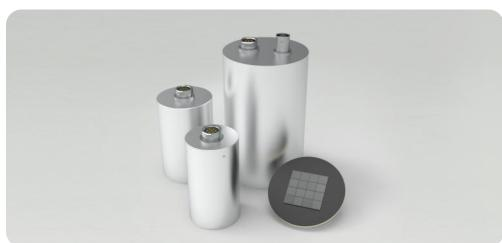
The ECB-D25H25SIPM01 spectroscopic detector is a highly integrated detector containing a 1-inch CeBr<sub>3</sub>, silicon photomultiplier (SiPM), summing circuit, preamplifier circuit, and temperature measurement circuit. It features excellent energy resolution, simple operation, compact size, and high reliability. It is widely used in industrial detection, radiological medicine, radiation detection, and other fields.
