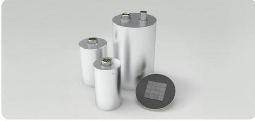
The ELBC-D50H50SIPM01 spectroscopic detector is a highly integrated detector containing a 2-inch LaBr<sub>3</sub>(Ce), silicon photomultiplier (SiPM), summing circuit, preamplifier circuit, and temperature measurement circuit. It features excellent energy resolution, simple operation, compact size, and high reliability. It is widely used in industrial detection, radiological medicine, radiation detection, and other fields.
