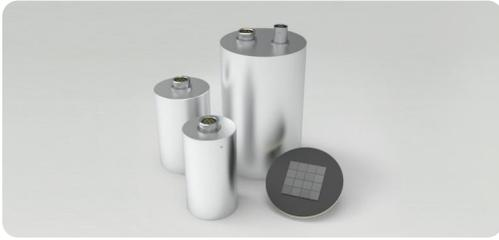
The ELBC-D38H38SIPM01 spectroscopic detector is a highly integrated detector containing a 1.5-inch LaBr<sub>3</sub>(Ce), silicon photomultiplier (SiPM), summing circuit, preamplifier circuit, and temperature measurement circuit. It features excellent energy resolution, simple operation, compact size, and high reliability. It is widely used in industrial detection, radiological medicine, radiation detection, and other fields.
