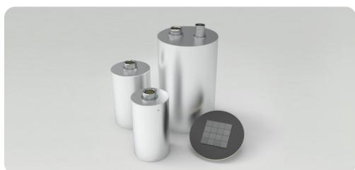
The ENAI-D50H50SIPM01 spectroscopic detector is a highly integrated detector containing a 2-inch NaI(Tl), silicon photomultiplier (SiPM), summing circuit, preamplifier circuit, and temperature measurement circuit. It features excellent energy resolution, simple operation, compact size, and high reliability. It is widely used in industrial detection, radiological medicine, radiation detection, and other fields.
