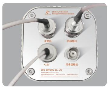
Model EP-AP2106 PMT dual readout preamplifier, can lead photomultiplier tube playing take pole signal and anode signal at the same time. Completes the simultaneous measurement of the energy spectrum signal and time signal by a single detector. According to the user's specific situation, it can choose whether to equip with the original precision high-voltage power supply or not.
