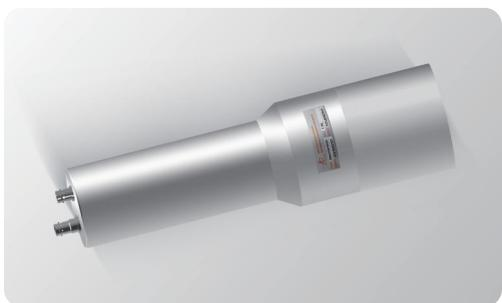
ENAI-D76H76VD01 scintillator detector is composed of a 3-inch Nal scintillator crystal, photomultiplier tube and voltage divider. Due to its high detection efficiency, good energy resolution, flexible matching, stable performance and easy to use, it is widely used in the fields of energy spectrum measurement analysis, building materials, food and other radioactive level analysis.
