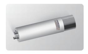
ENAI-D50H50VD01 scintillator detector is composed of a 2-inch Nal scintillator crystal, photomultiplier tube and voltage divider. Due to its high detection efficiency, good energy resolution, flexible matching, stable performance and easy to use, it is widely used in energy spectrum measurement and analysis, food testing, densitometry and other fields.
