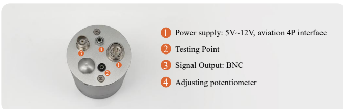
High voltage divider socket
