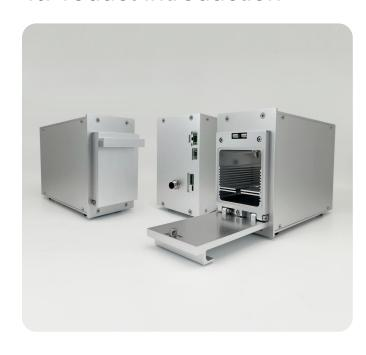
EPIC-APD8127 Alpha Spectrometer is a single-channel PIPS semiconductor detector Alpha Spectrometer designed to support chambers with up to 1200mm² and up to 3000mm² detectors, which can be applied to qualitative and quantitative analysis of Alpha particles. Includes vacuum measurement chamber, PIPS detector, preamplifier circuit board, high and low voltage power supply and single channel control board, high performance digital multichannel board, vacuum sensor.
