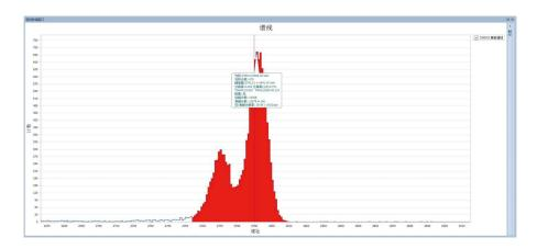
The results of the Pu238 resolution test by EPIC-APD8127 Alpha spectrometer are shown in Fig. The energy resolution of the tested  $450 \text{mm}^2$  PIPS detector is up to 23.623 keV @ 5499 keV.
