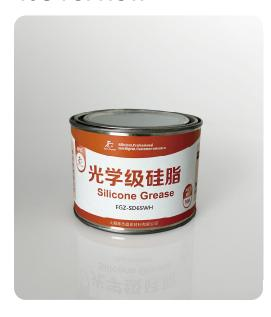
EGZ-SD65WH is a clear, colorless, silicone, optical coupling compound that features excellent light transmission and low evaporation and bleed at 25 degree C, and it has a specific gravity of 1.12 and 1.467 index of refraction. EGZ-SD65WH is for optical coupling of photosensors to scintillators and light guides, for example the coupling of photomultiplier tubes. Projector picture tube filling, oil exploration tools, electronic components, optical fiber bonding, filling and fixing, etc.
